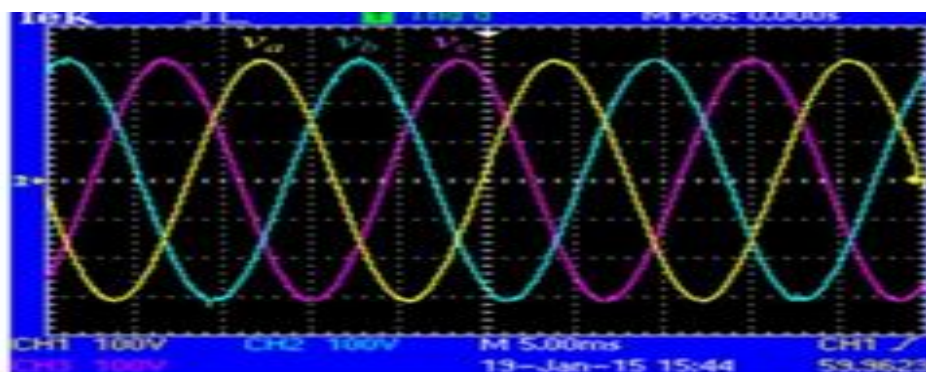
Fig 5.PCC Voltage Compensation for linear loads
