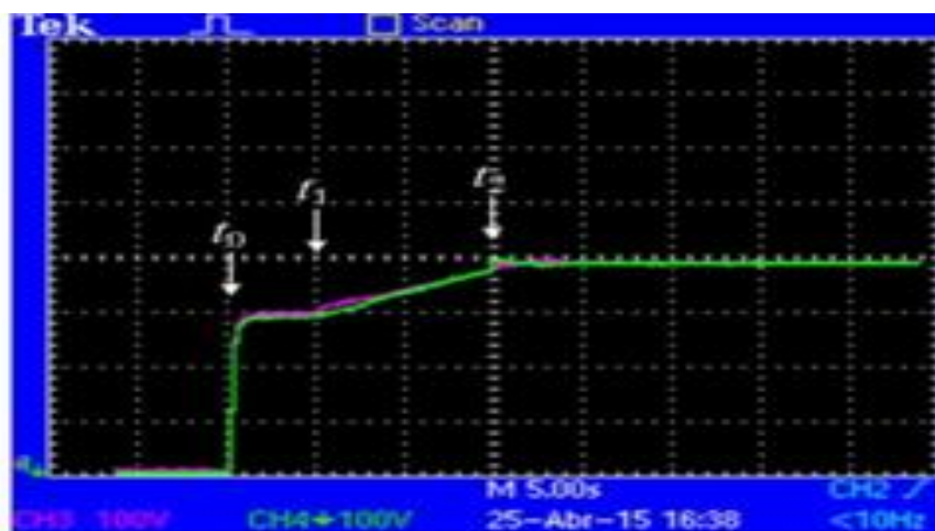
Fig 4.DC Bus Voltage during STATCOM Initialisation
